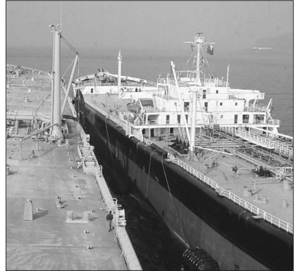
Having made contact the helm of the smaller tanker is placed hard to port to secure the bows.
