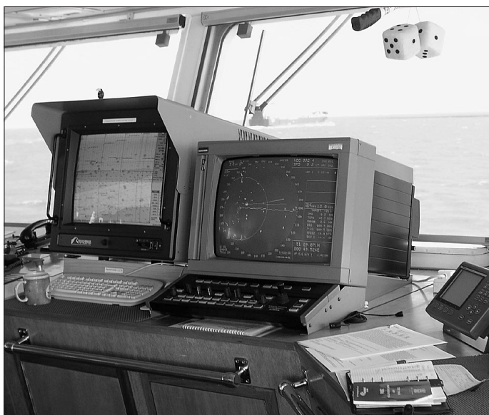
Picture 5. ENC, Radar and IAS (plus essential coffe mug - pink fluffy dice optional!)
