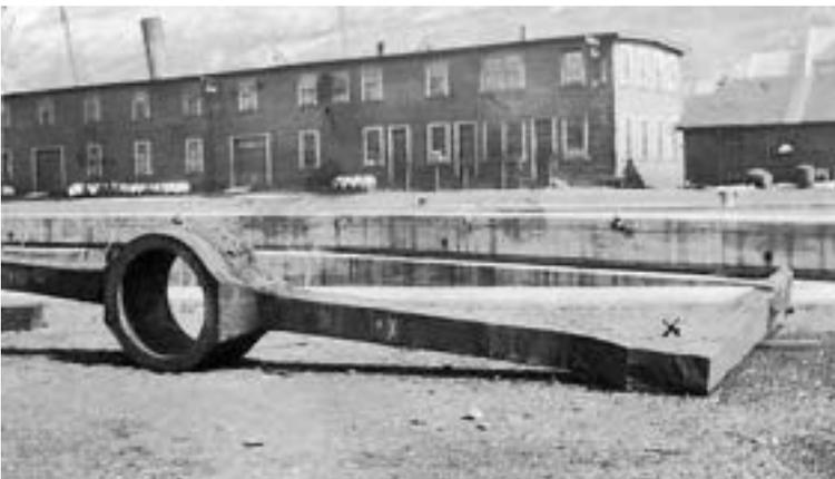
CAIRNGOWAN'S fractured stern frame. at St. Johns N.F. Taken on 20<sup>th</sup> April.1929. (Cross marks fracture).
