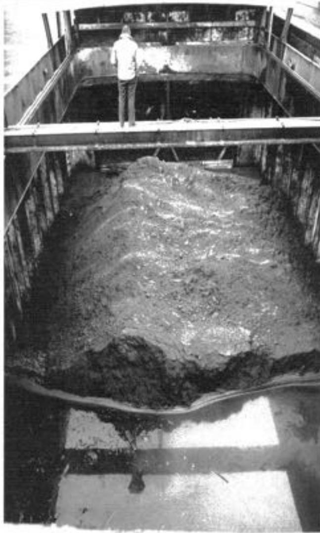
Photographs show Cairnover in Esbjerg. Surveyors said that the water could be pumped from the top of the cargo but ships officers, who had been carrying out their own tests of moisture content disagreed as did company surveyors so eventually all the cargo had to be discharged. This became a lengthy undertaking since bad weather, snowfalls etc, delayed the removal of the necessary machinery. Eventually all cargo was removed and the vessel continued trading
